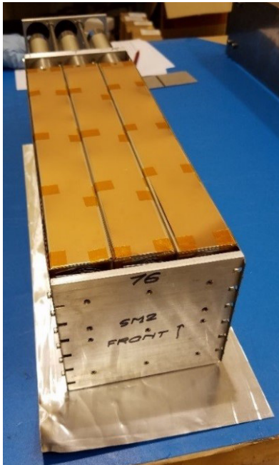
FIG. 4. Assembled supermodule just before step of wrapping bottom in aluminum foil.
