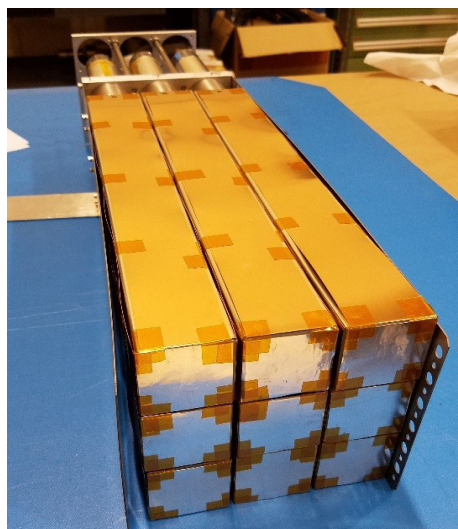
FIG. 3. Lead glass blocks in a 3X3 matrix in the support frame.
